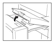
4 Remove any paper, and then close the cover of the horizontal transport unit.
